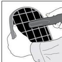
Clean the filter using a vacuum cleaner on a low power. Replace the filter cartridge onto the rear panel.
